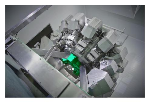
The MultiCheck detects the foreign objects when the product stream drops off. Several cameras take pictures simultaneously from different positions. (Photo: © CLK GmbH)
