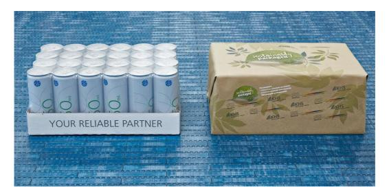
Whether wrapparound, tray or pad, with or without film wrapping or wrapping in paper - the Innopack processes a wide variety of secondary packaging. (Photo: © KHS)
