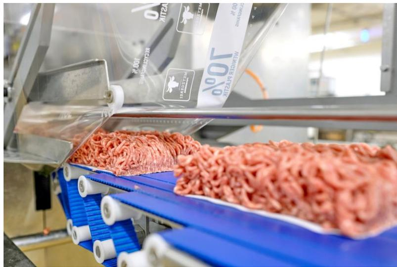
To optimise the flow-pack packaging process, the folding geometry of the film was changed. (Photo: © Ingo Jensen/Ulma)
